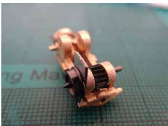
Figure 2: Fitting the wheels and gears
