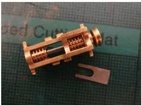
Figure 1: Chassis with layshaft fitted.
